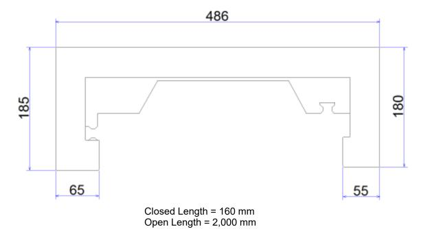
Note: Dimensions are in MM and are for identification purposes only and not for inspection.
